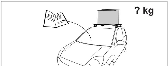
When these roof racks are to be used on a vehicle that is driven off sealed roads, the manufacturer maximum roof load rating (to be found in the vehicles User Manual) should be **halved**. Do not forget to subtract 7.5kg from your maximum carrying capacity due to the weight of the crossbars and legs.
