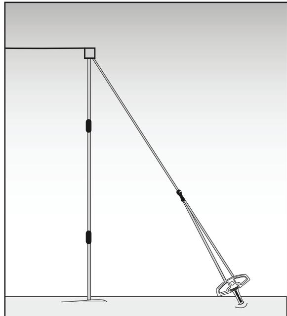
We recommend setting the angle of the Sand Screw to be in line with the attaching rope.
